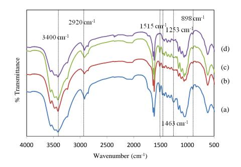
**Figure 1:** FT-IR spectra of (a) untreated SCB, (b) steam exploded SCB, (c) steam exploded SCB with xylanase treated and (d) bleached fiber
